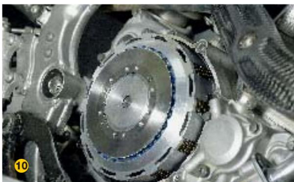
10-11 | FIXER SOIGNEUSEMENT LE PLATEAU DE FERMETURE AVEC LES VIS M3 TORX. LE COUVERCLE DE L'EMBRAYAGE PEUT ENSUITE ÊTRE REPOSÉ
