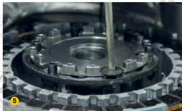
5 | AVEC SOIN, ON REMPLACE LES BOULONS PAR DES VIS À TÊTE PLATE MOYENNEMENT SERRÉES
