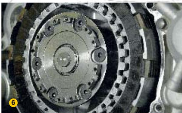
6 | QUAND LES 6 VIS SONT POSÉES, LE AUSRUECKER EST MIS EN PLACE (AU CENTRE DE LA BASE)
